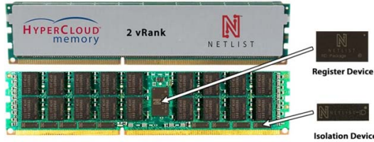
Figure 5. HyperCloud™ Memory provides load reduction and rank multiplication for high speed, high density memory.
